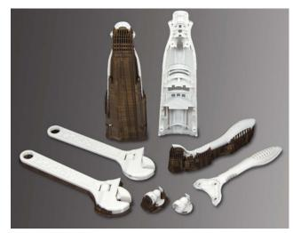
to 0.013 inch [.330 mm], depending on the system.) The print head moves in X-Y coordinates, and the modeling base moves down the Z axis as the model and its support material are built from the bottom up.
